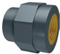
BR PVC-U-Rotguss/Messing/LFB Übergang IG-zy1 grau BR PVC-U-Bronze/Brass/LFB Transition female-thread-cyl grey
