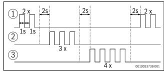
Fig. 12 Flashing patterns
