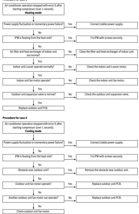
Check the cause due to PCB or another parts.
