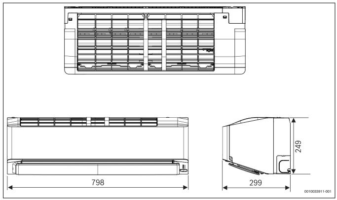
Fig. 1 Indoor unit dimensions (in mm)
