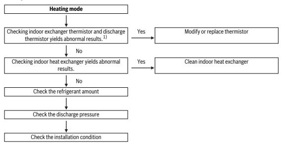
1) Check to make sure thermistors are installed in correct portions. See section 4.4 "Thermistor Temperature Characteristics".
