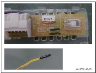
Fig. 131 Room temperature thermistor
