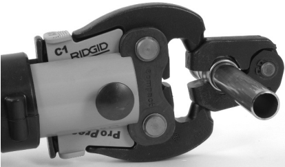
Figure 10 – Attaching Actuator to Press Ring
