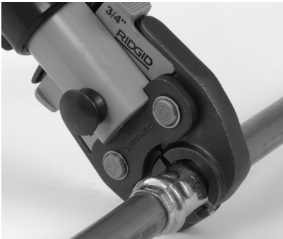
Figure 7 – Placing Scissor-Style Jaws Around Fitting
