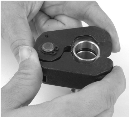
Figure 9 – Installing Press Ring onto Fitting
