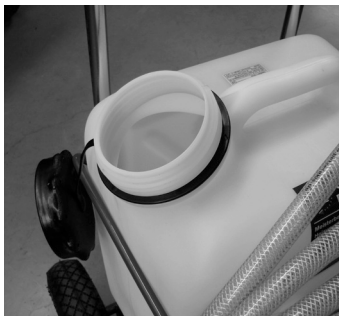
5. Open tank lid to ensure the circulation of the air.
