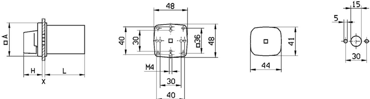
A=48mm, H=27mm, Xmax=4mm, L=57mm
