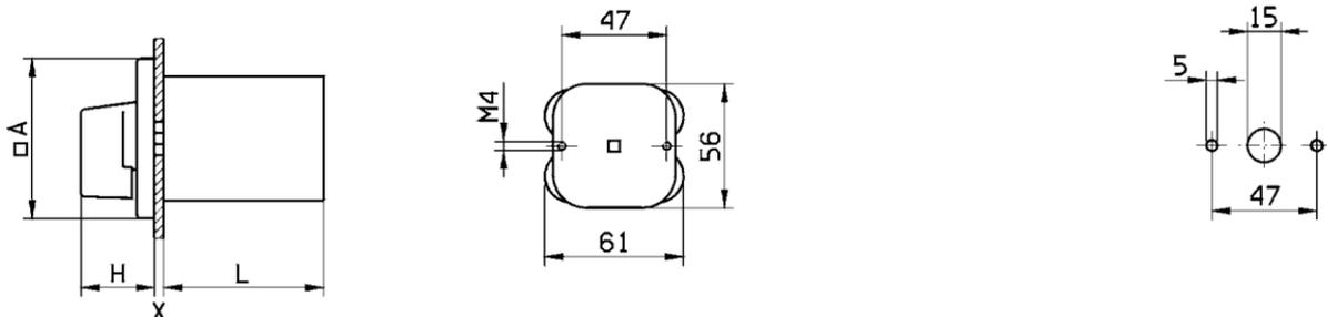
A=72mm, H=34mm, Xmax=4mm, L=92mm
