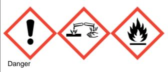
H315-Causes skin irritation. H318-Causes serious eye damage. H336-May cause drowsiness or dizziness. H412-Harmful to aquatic life with long lasting effects. H222-Extremely flammable aerosol. H229-Pressurised container: May burst if heated.
