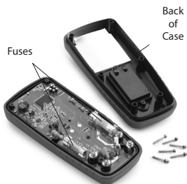
Figure 9 – Removing Back of Multimeter Case
