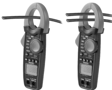
Figure 8 – Correct Way of Current Measurement
