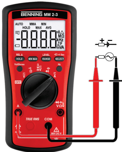
Figure 10: Current or frequency measurement
