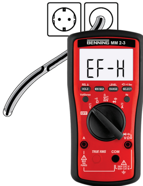
Figure 14: Non-contact phase testing
